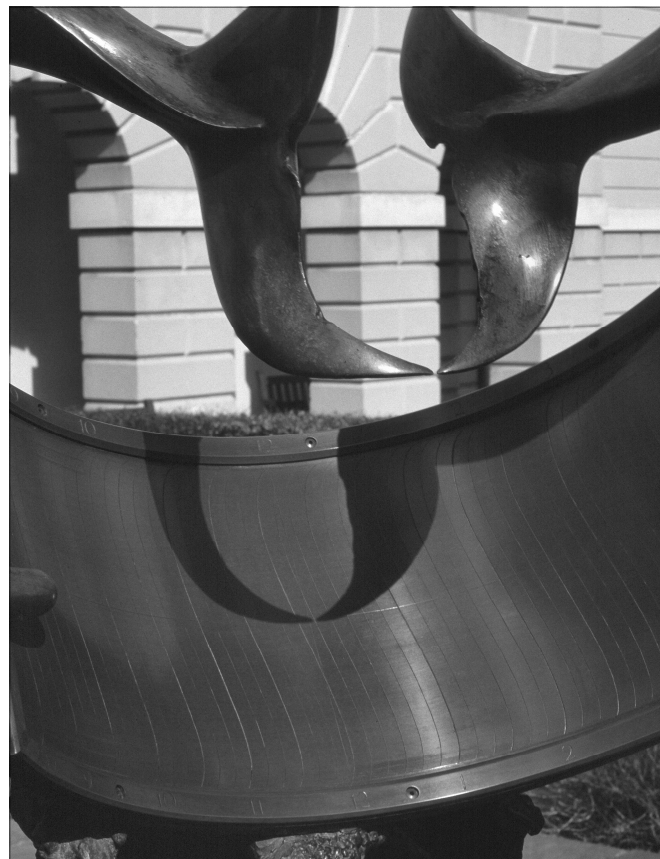
Fig. 37. Detail of the 'Dolphin' sundial at the National Maritime Museum at Greenwich. The gap between the shadows of the dolphins' tails, passing over the analemmic hour-lines, indicates the time to within some 30 seconds. The time indicated is 12:10 GMT.
