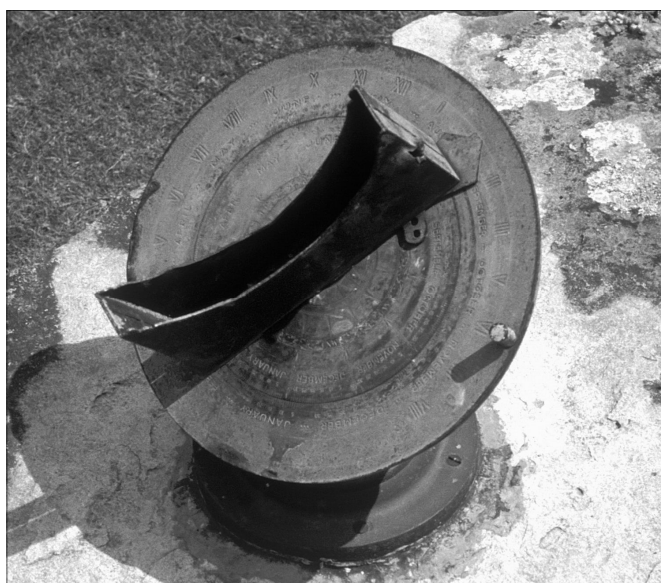
Fig. 19. Pilkington's mean-time sundial, the 'Sol Horometer', patented in 1911.
