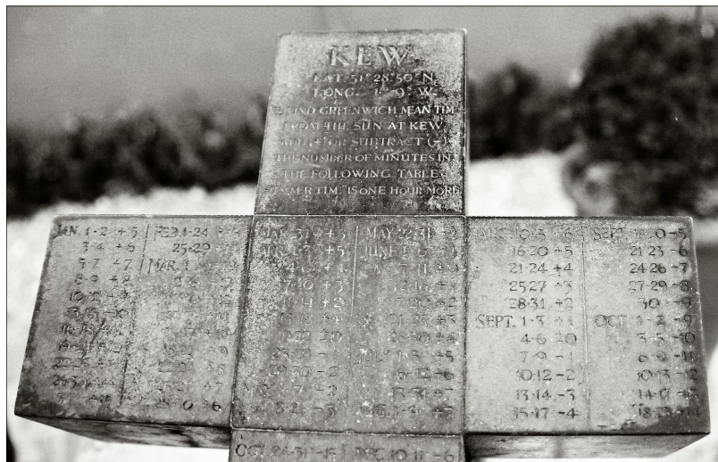
Fig. 5. The north facing side with the tabular equation of time and instructions.
