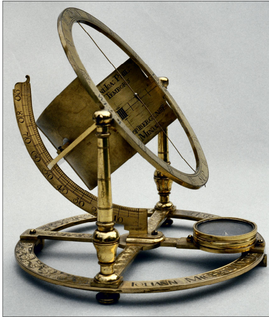
Fig. 29 (far left). The portable universal equinoctial mean-time sundial, made by Johann Michael Vogler for Johann Philipp von Wurzelbau c. 1716, in the gnomonical collection of the National Maritime Museum at Greenwich.
